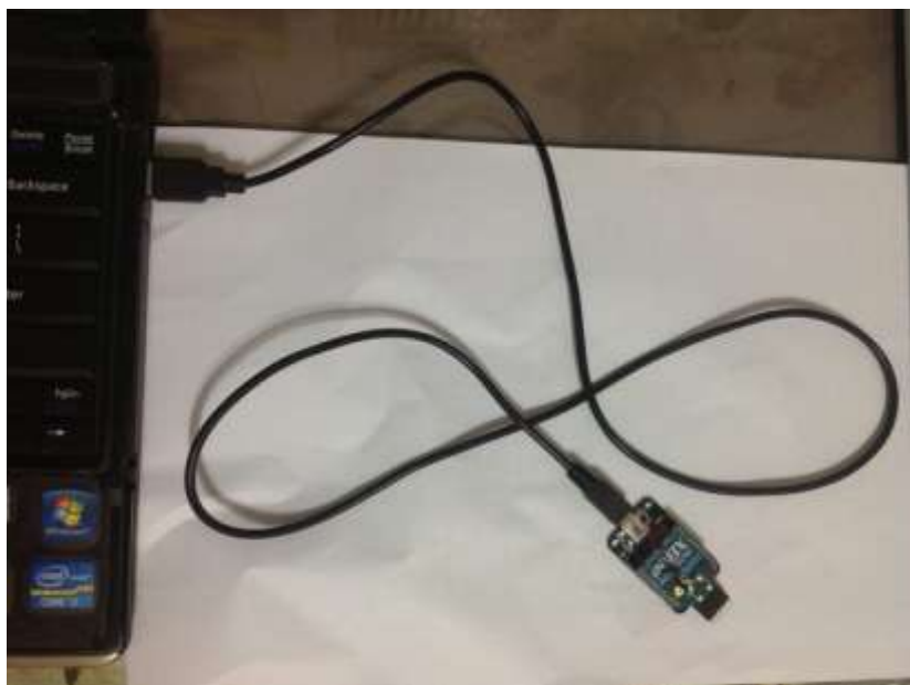
Figure 5.1: Connection of XBee to PC with USB Cable
